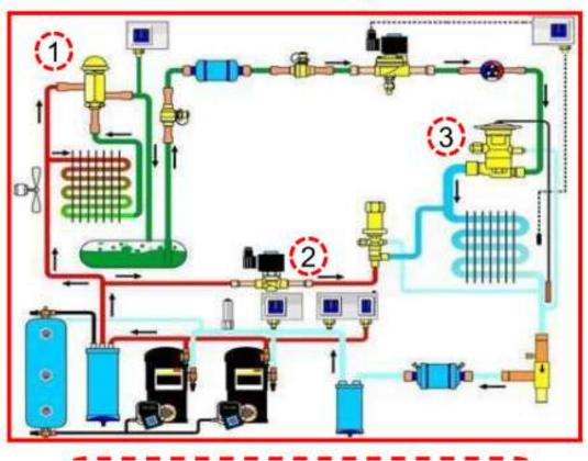
Reducing Energy use: Floating Head Pressure & Efficient Condensing
